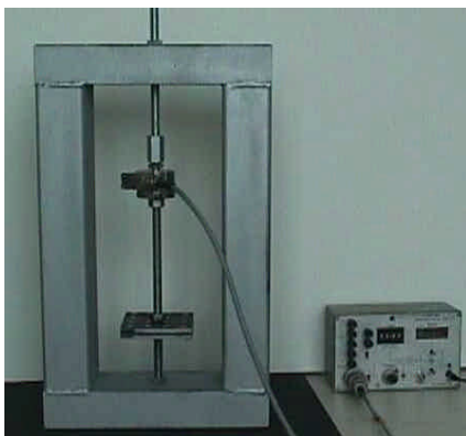
Fig.18 Testing arrangement for the particle tensile strength
